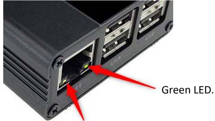
Lets look at the Green LED on the back, visible through the same slot in the case as the Red LED on the back.
